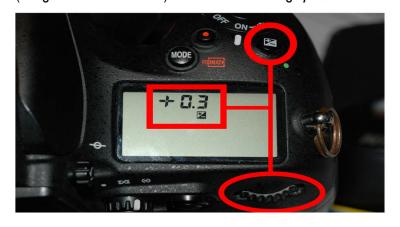
While this can be compensated for in post-processing, the camera's auto-exposure can be manually adjusted using the exposure compensation button (or menu). Most DSLRs will allow you to lighten (positive compensation) or darken (negative compensation) the exposure relative to the camera's auto-setting. Exposure compensation (EC) can typically be set up to  $\pm 5$  EV (or 'stops') in  $\frac{1}{2}$  or  $\boxed{EV}$  steps. EC is most effective when used with spot or centre-weighed metering modes
