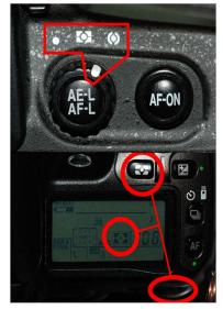
**Matrix:** the camera meters a wide area (more or less the whole fame) and sets the exposure according to the distribution of colour, composition and 3D distance (if the lens supports it). The whole frame area may be given equal weight, or the central part of the frame may be given a little more weight than the edges, depending on the camera design. Matrix mode is most useful for wide-area shots such as landscapes, where a balance of exposure over the whole frame is required.
