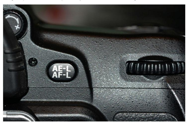
DSLRs will also usually have a dedicated AE-L/AF-L button (as above) which can be set up in the menu to act on exposure alone (AE-L), focus only (AF-L) or both (default). In AE-L mode, when this button is pressed (depending on the camera, a singe press may hold the setting, or you may have to keep pressing it), the initial exposure will be maintained, allowing re-composition and possible refocussing by releasing the shutter button and taking the shot when ready again.
